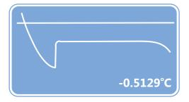
A graph charting the actual freezing point curve, in real-time for each sample tested, is displayed on the readout display. This provides in-depth insight helpful for a multitude of purposes, including troubleshooting and Research & Development.
